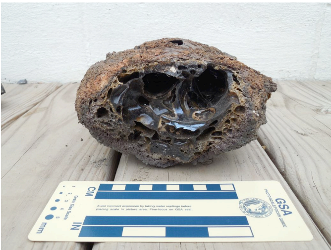
Figure 5. Section of the Rebersburg fulgurite measuring 15 by 10 cm in cross section and having 3- to 4-cm vesicles. This specimen also has an outer 2-cm zone having smaller vesicles.
