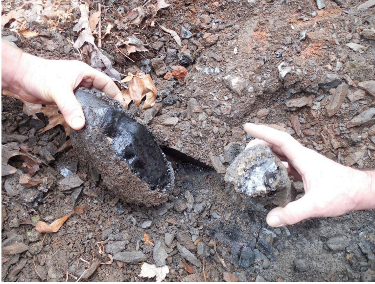
Figure 3. Solid glass sample from the central axis of the Rebersburg fulgurite measuring 17 by 6 cm in cross section.
