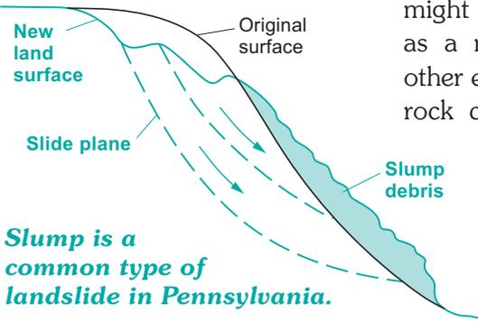
**Slump is a common type of landslide in Pennsylvania.**
