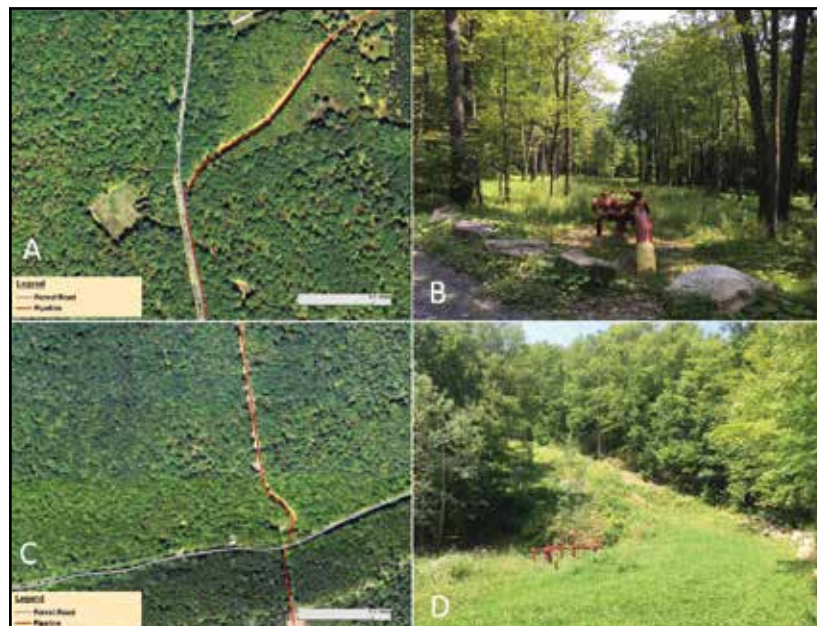
Figure 6.18. Two examples of pipeline rights-of-way with strategic bends to reduce line-of-sight from forest roads. Note how a relatively slight bend (seen in aerial imagery) creates a reduced line-of-sight of non-forested area (seen in photos)
