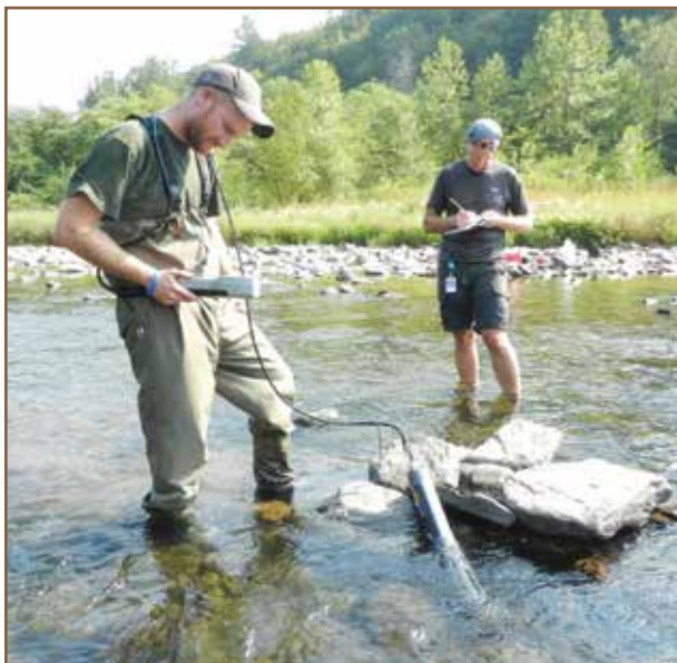
A continuous in-stream monitoring device utilized by PA DEP, called a "Sonde", shown here during a maintenance visit.
