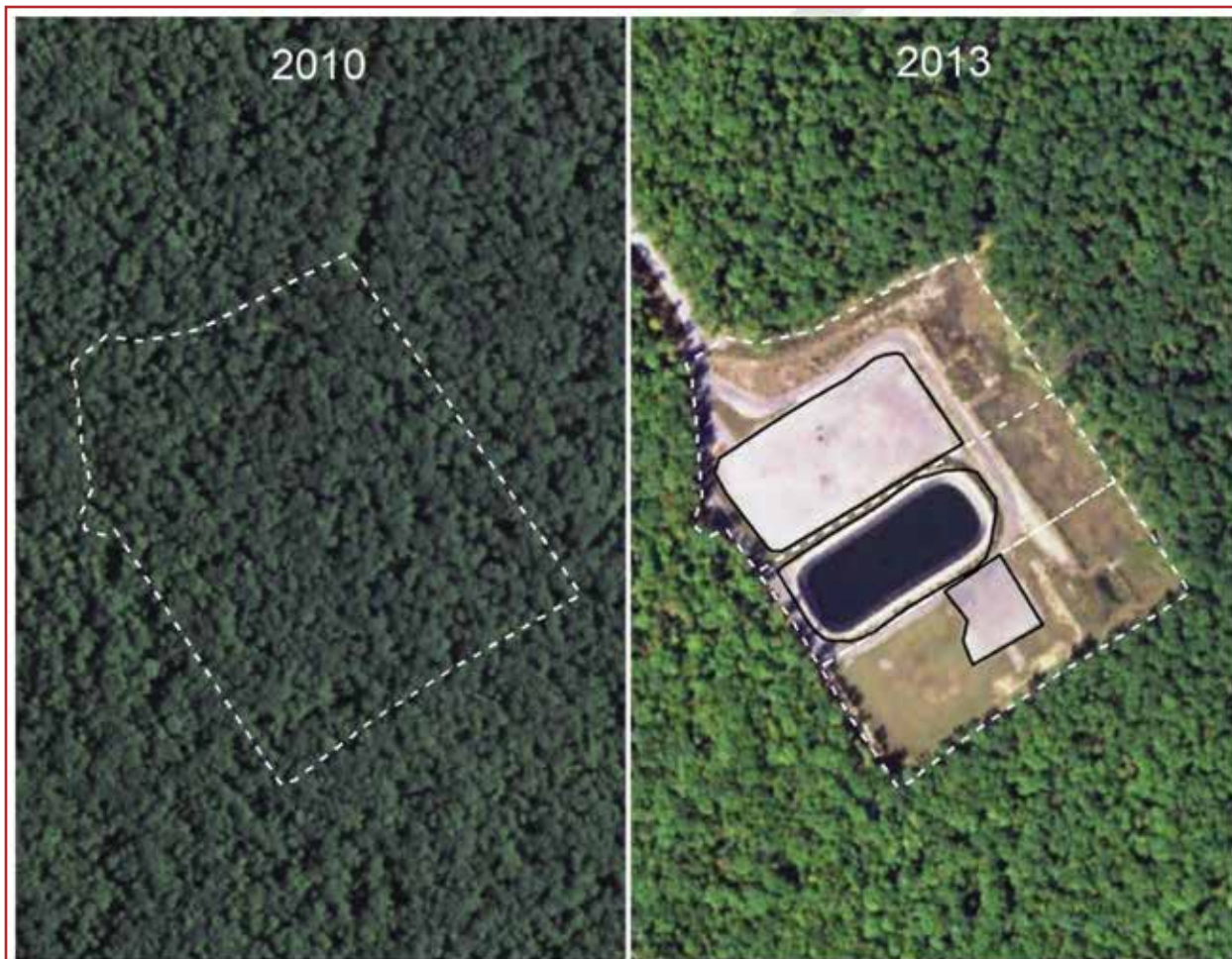
Figure 4.12. Illustration of how the digitally represented pad boundaries have been corrected over time. In the first report the latest aerial image for this site (left side) was taken prior to construction. The actual pad boundary, number of pads, and limit of clearance is unknown. Therefore, this site was classified as one well pad. The well pad limit of clearance (white dashed line) was used as the pad acreage. In 2013 (right side), a new aerial image was available, and three separate pad types were clearly visible (in black); a well pad, a freshwater impoundment, and a storage pad. Each of these pads is given its own limit of clearance (white dashed line). This results in more pads and less total pad acreage/
