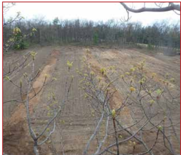
Aerial view of mock pad site with four soil treatments – from left to right: (1) topsoil spread over compacted rock and subsoil, (2) topsoil spread over compacted subsoil, (3) 8” ripping, and (4) 20” ripping.
