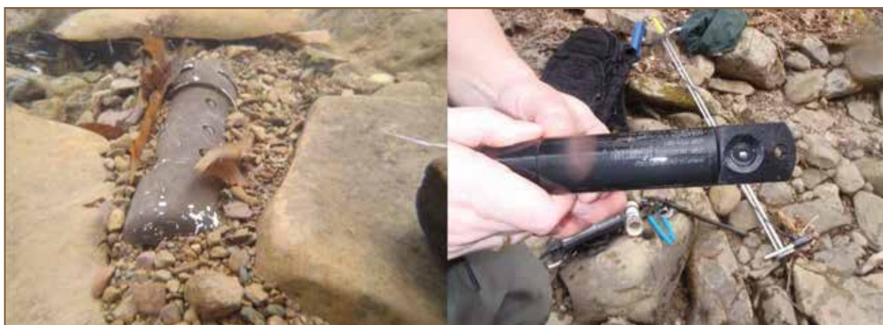
A continuous in-stream monitoring device utilized by the bureau, called a “Hobo”, shown here deployed in a stream and out for cleaning during a maintenance visit.
