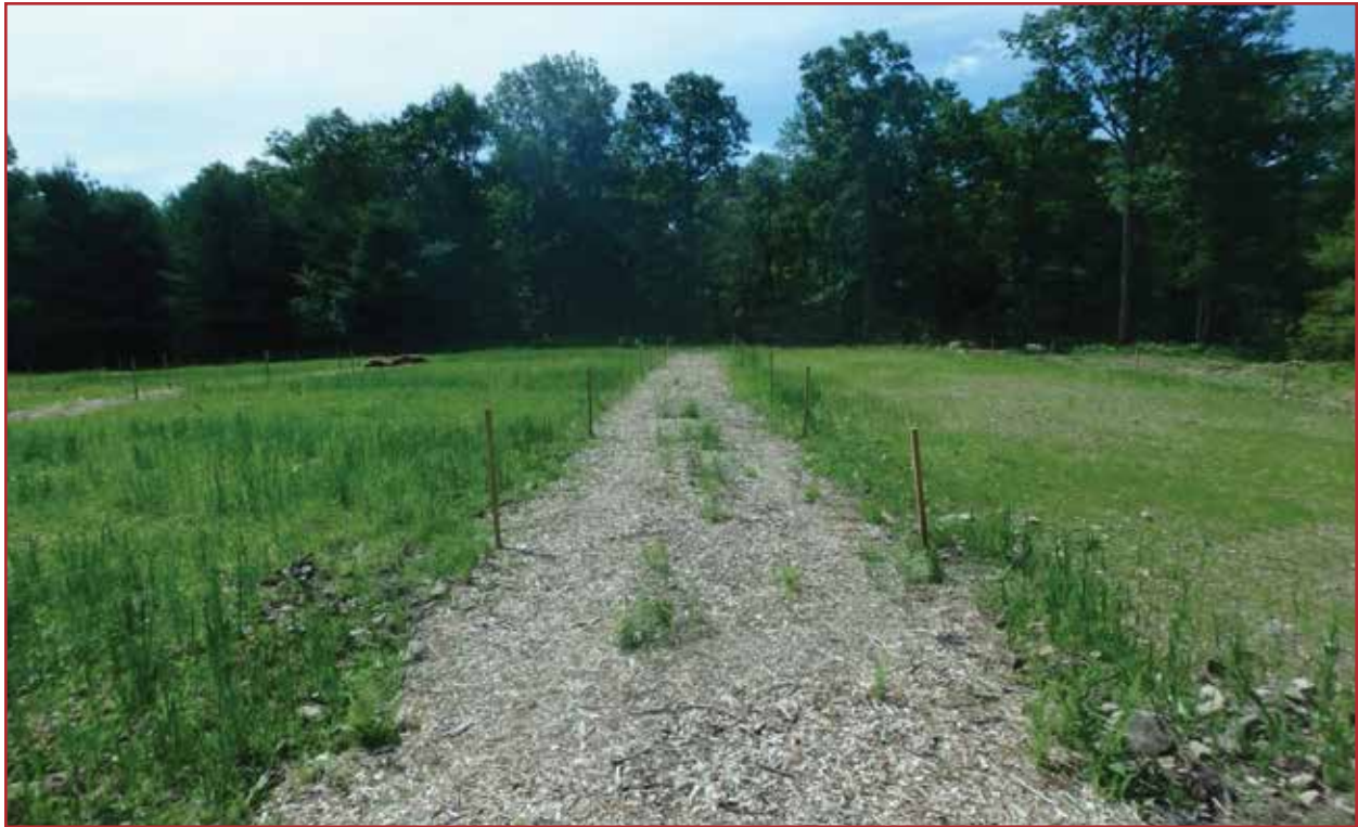
Initial establishment of seed mixes 45 days after planting. Topsoil spread over compact subsoil treatment (on left) versus topsoil spread over compact rock and subsoil (on right). Note increased height of grasses on left.
