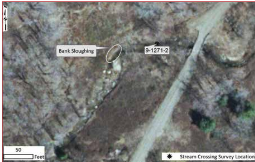
Figure 4.19. A 2006 aerial photograph of the power line right-of-way adjacent to the crossing in the Moshannon State Forest. This photograph was taken 5 years prior to the installation of the pipeline. Bank sloughing that was detected in the 2016 assessment is also seen in this photograph.
