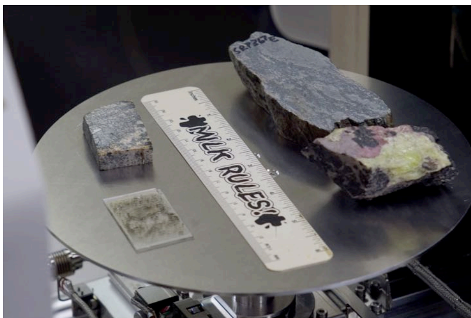
Figure 2. Our largest sample holder (200 mm [8 in.]) can accommodate many samples at one time, including (in clockwise order from bottom left) petrographic thin sections, slide billets, rock slabs, rough rock samples, and plastic rulers with unruly messages. What is shown is not an optimal analysis strategy; analysis is most ideal if the samples in the same batch are similar in height. ( Back to text )
