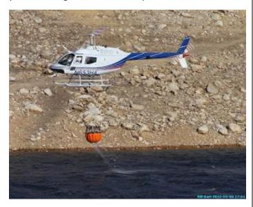
Helicopters are useful to combat hot-spotting, reconnoiter the fire, walk resources into a fire that they can't find, or help map the fire. They can also maneuver in areas that tankers cannot. The Type 3s can drop 90 gallons of water at a time, while the Type 2s can drop 300 gallons at a time and can load from a water source closer to the incident than an airport.
