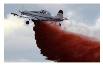
The other useful thing that air tankers can do is change the level of their drop, and split loads. There are four levels that the gate can open: Level 1 is for grass and light fuels, the gate doesn't open far; level 2, then level 3, and level 4 is wide open for heavy timber/fuels. Splitting loads means that they close the gate when about half of the retardant is left in the hopper. This can be used to your advantage to hit different spots on the fire.
