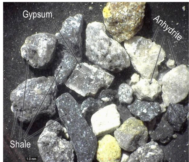
Figure 5. Anhydrite, shale, and trace gypsum (variety selenite) in the Salina Formation (6,710 ft measured depth).
