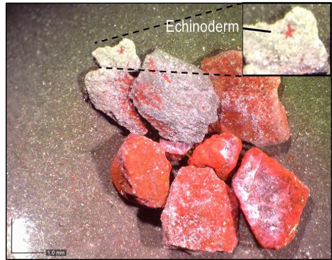
Figure 7. Trenton Limestone (12,110 ft measured depth) after treatment with Alizarin Red S. Likely echinoderm fossil (red-stained star) in the upper left cutting (enlargement of cutting shown in upper right).
