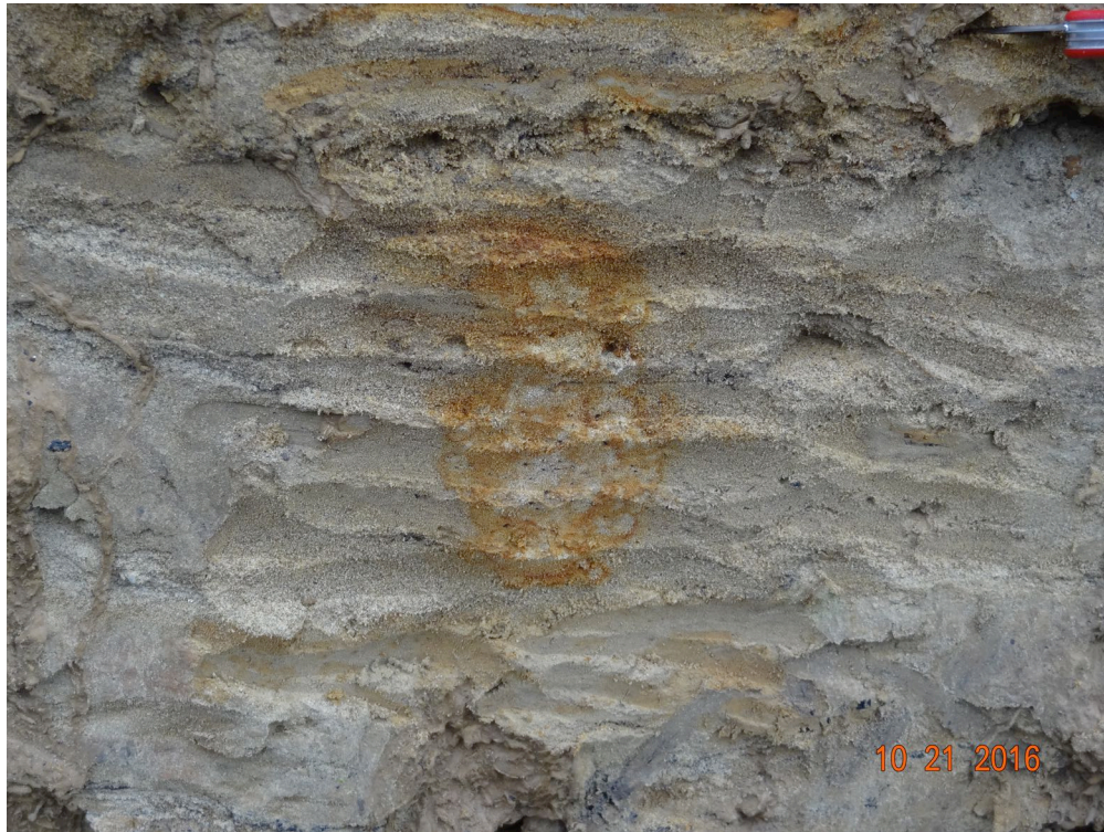
Figure 5. Photograph of fine sand and silt of the deltaic sediments, probably similar to those encountered during dam construction. This photograph was taken at an excavation for the sewage-treatment plant about 1/10 mile west of the south end of the dam. Pocket knife in upper right corner for scale.
