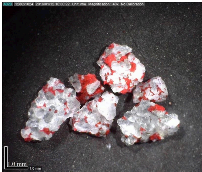
Figure 4. Oriskany Sandstone cuttings (5,680 ft measured depth) from the Harry Dewey #1 well after treatment with Alizarin Red S solution. Abundant calcite cement (red staining) is apparent between the sandstone clasts.
