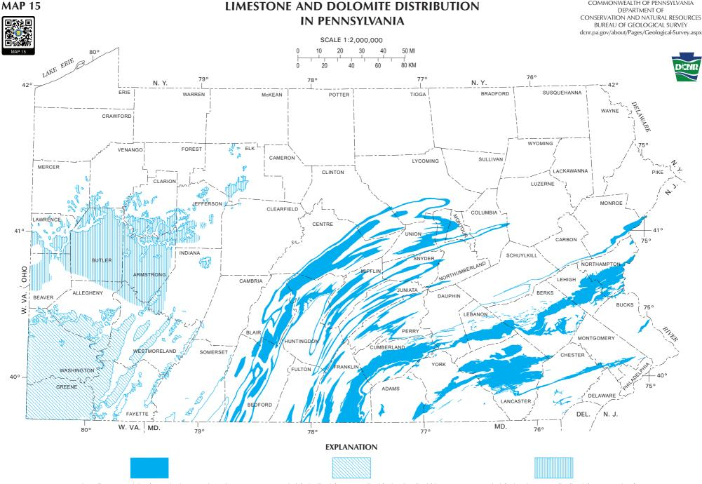
Area where limestone, dolomite, or both are at the suface. Layers are usually strongly folded and steeply dipping. Includes economically important high-calcium limestones of the Kinzers, Annville, Benner, and Keyser Formations and the Cockeysville Marble, as well as the high-magnesian dolomites of the Ledger Formation and the Cockeysville Marble. This area is most susceptible to sinkhole development.
