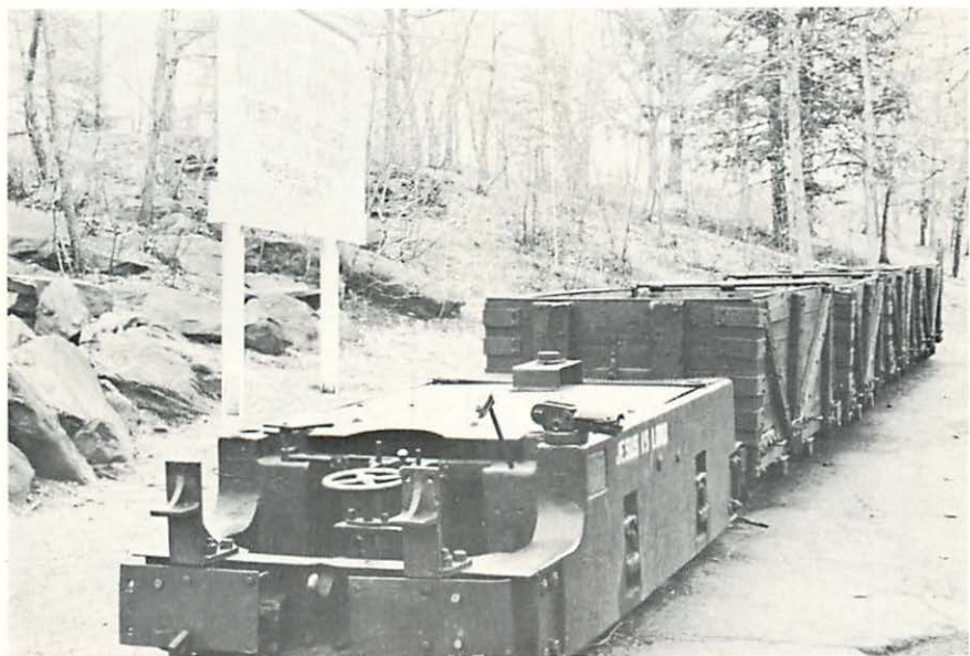
Fig. 3. Motor used to pull loaded coal cars from the mines.
