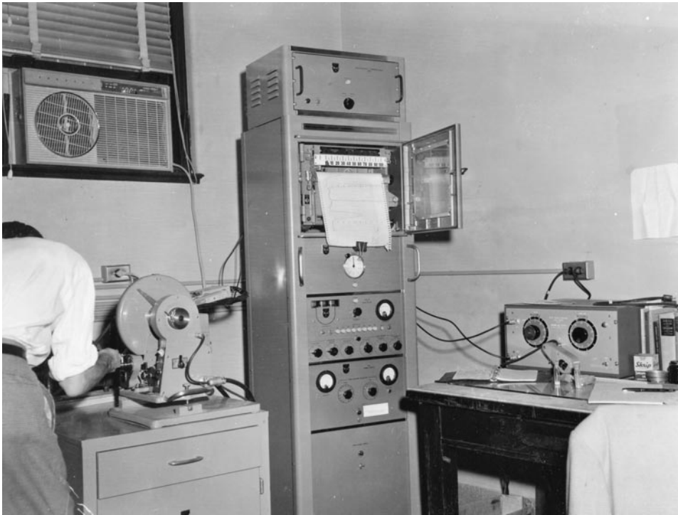
Figure 8. Davis M. Lapham, Survey mineralogist, working in 1958 with the Survey's first X-ray diffractometer, acquired two years earlier.
