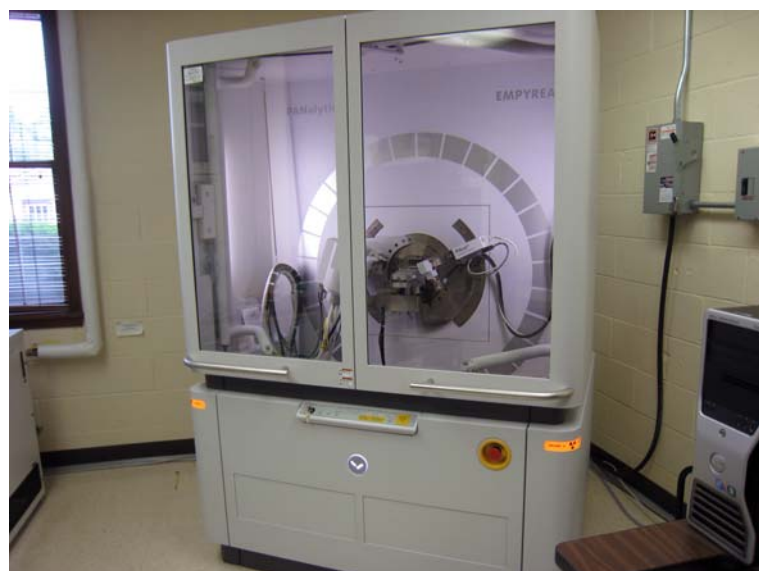
Figure 2. The bureau recently replaced its aging X-ray diffractometer with this up-to-date unit.
