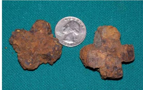
Figure 3. X-shaped drill bits were placed at the end of a rod, which was hammered by hand with a quarter turn between each strike. In this fashion, workers drilled holes in the rock to insert explosives. As the bits became dull, they were discarded.
