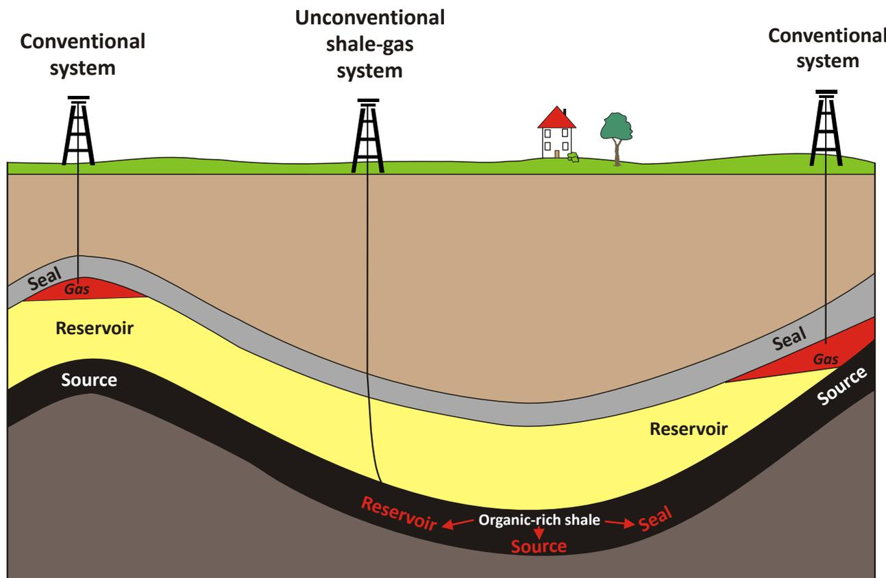
Figure 2. Schematic diagram illustrating the elements of a conventional petroleum system and an unconventional shale-gas petroleum system. Modified from Schmoker and Oscarson (1995).
