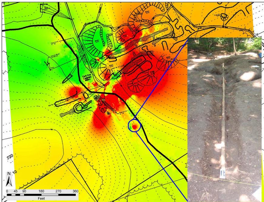
Figure 4. Map showing the magnetic anomaly in red (circled) and photograph of the excavated rail (right) at the York Iron Company mine site.
