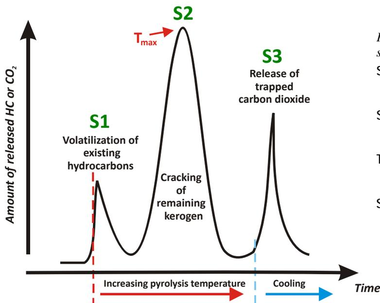
Figure 4. Typical Rock-Eval pyrolysis output graph showing S1, S2, S3, and Tmax.
