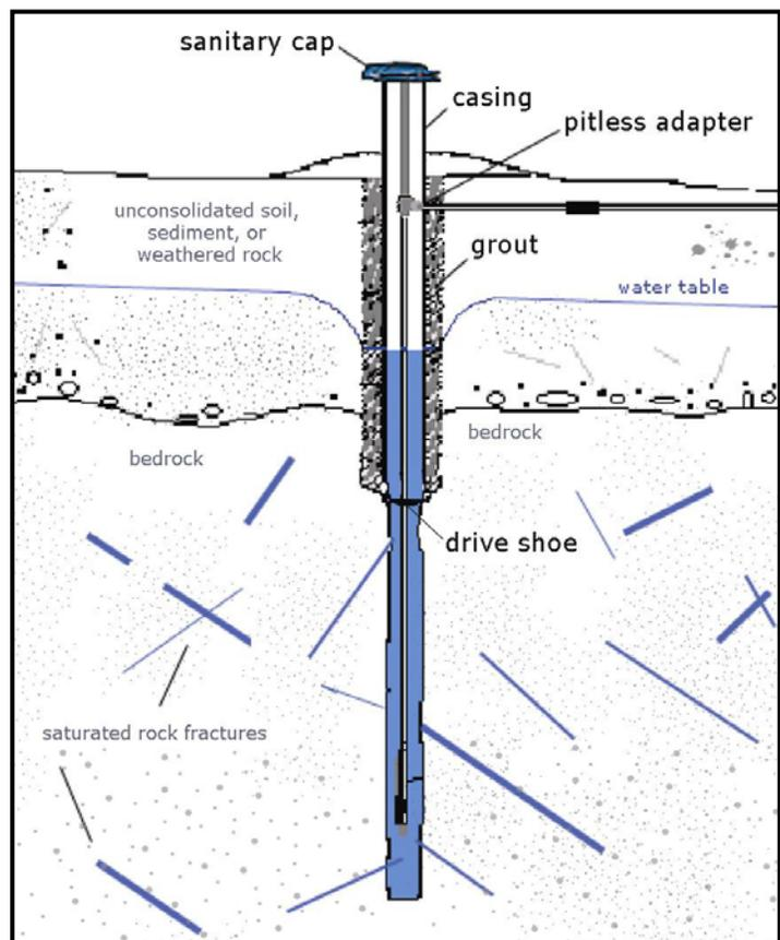
*Figure from the fact sheet showing components of an open-hole water well located in bedrock.*
