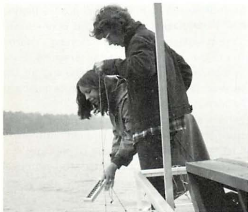
Girls using forel water comparator and secchi disk. Prince Gallitzin State Park.
