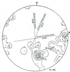
strike joints along a kink fold at the apex of the head scarp (Figures 4 and 5). The southeast side was the open face of the roadcut. The slide surface stepped down slightly from the top to the bottom of the thin siltstone bed in the northeast part of the slide area (Figure 5). Because the pre-split slope cuts obliquely across the strike of bedding, the slide mass actually rotated about 40 degrees to the southeast toward its unbound side as it moved off the slope.
