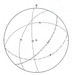
Figure 4. Stereogram (equal-area lower hemisphere projection) of major discontinuity surfaces of the rockslide. Bedding: B, N80E/-40SE (failure surface). Joints:  $J_s$  (strike), N78E/45NW;  $J_d$  (dip), N6W/80W;  $J_o$  (oblique), N21E/-52NW. The cut face shown (N40E at  $\frac{1}{2}$  to 1, or 63 degrees) is the design cut slope prior to failure.
