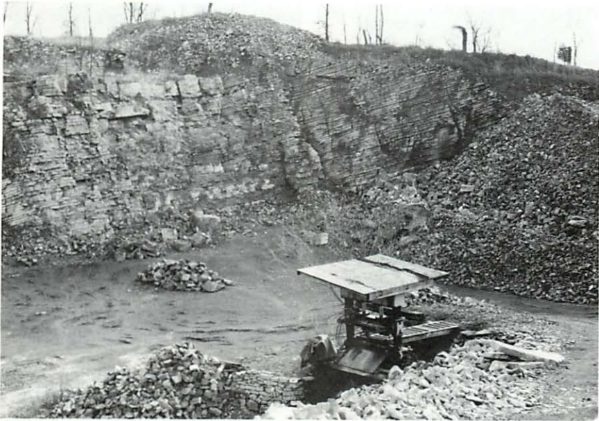
Figure 1. View of the active Caretti Quarry looking to the southeast. Note the flaggy to slabby bedding. Quarry waste is being backfilled to the west (right). Hydraulic rock cutter is in the foreground. Stockpile on floor of quarry is about 9 tons of random-size quarry-run.
