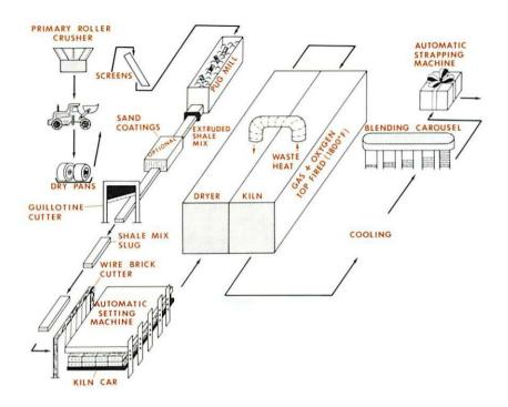
Figure 3. Simplified flow chart of the brick making process at Watsontown Brick Co., Watsontown, Pennsylvania.
