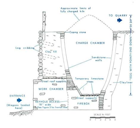
Fig. 2 Cross-section of the Arthur L. Long lime kiln. The firebox, shown here in longitudinal section, is used intially to ignite the charge above the steel supports and temporary limestone stops. The keyhole access provides draft to the firebox and charge chamber, and is used to extract the lump lime after the completed burn. Kiln is shown uncharged.
