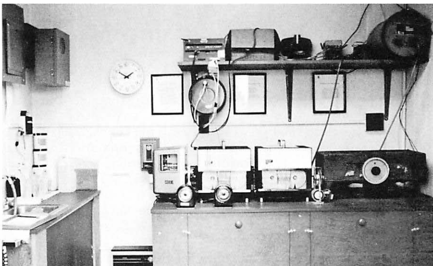
Instruments in Susquehanna River monitoring station at Harrisburg; includes automated LANDSAT satellite data collection system, electrical tapes, and recorders.
