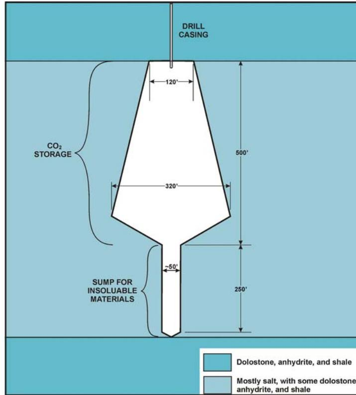
**Figure 4.1-3. Schematic diagram of a potential leached salt cavern in north-central Pennsylvania.**<sup>F15</sup>
