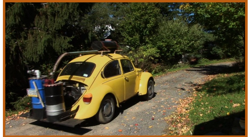
Gary Gilmore’s retooled VW, fueled by wood chips
