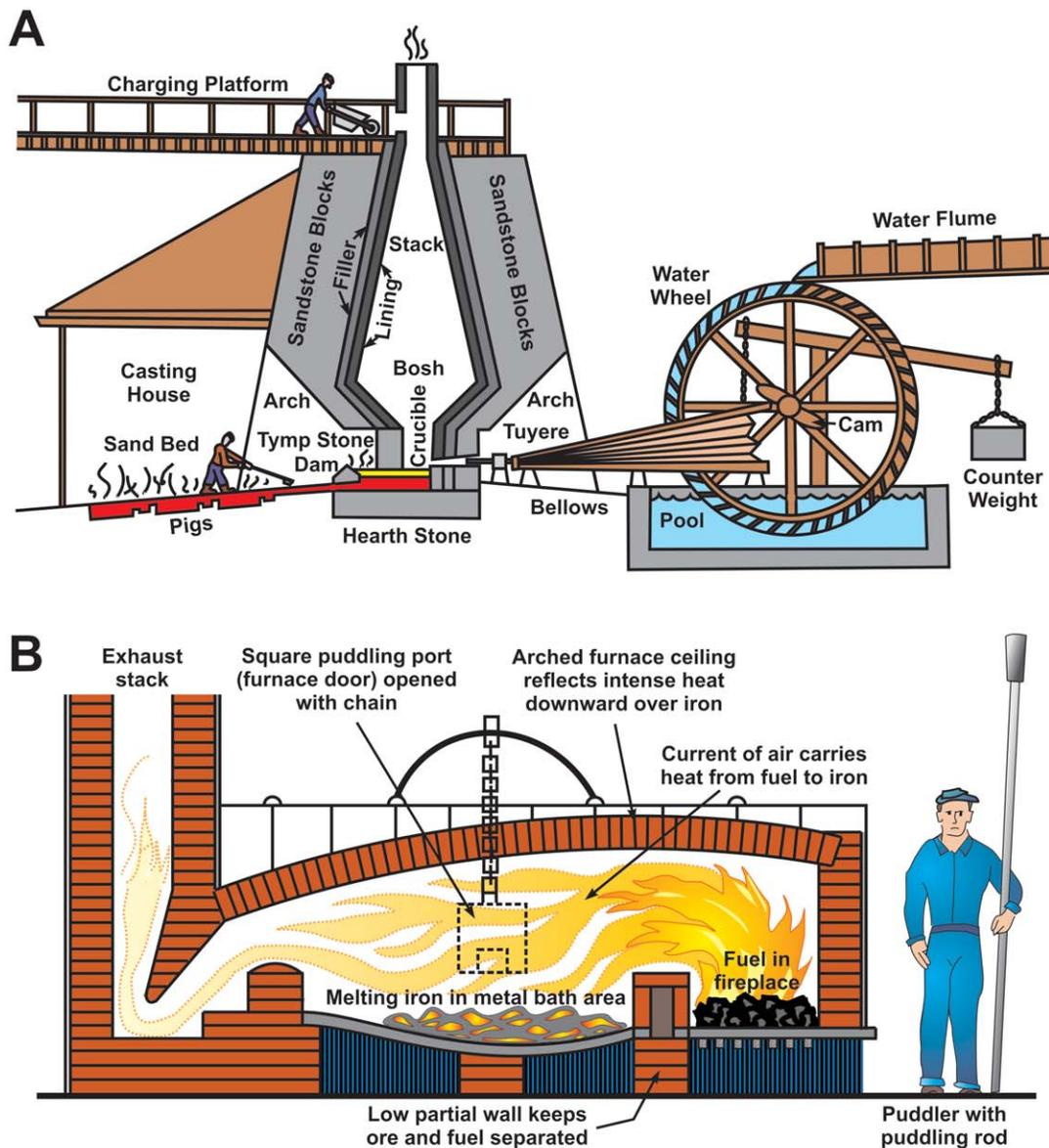
Figure 3. A. A typical charcoal blast furnace (from Samways and others, 2014). B. A puddling furnace (modified from Samways, 2016). See text for explanation of how these furnaces worked. Not to scale. Both illustrations based on drawings by David J. Vater.
